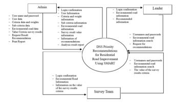
Fig. 3. Context Diagram of System for recommending priority for road improvement
