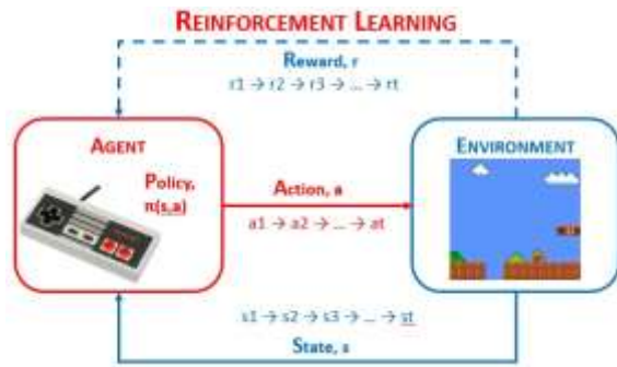
Fig. 3. RL agent in the state s , and then performing action a based on policy \pi , resulting in reward r and new state s' . (Components of RL)
