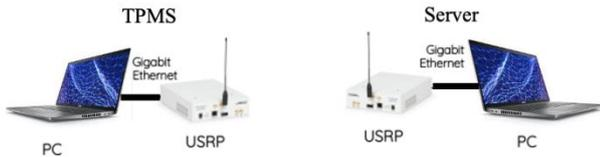
Fig. 8. Hardware configuration
