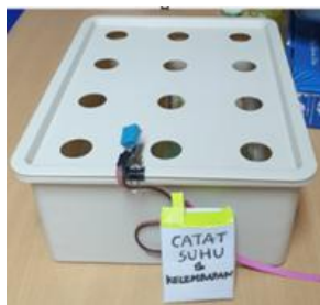
Fig. 7. DHT11 sensor and ESP8266 Node MCU wrapped
