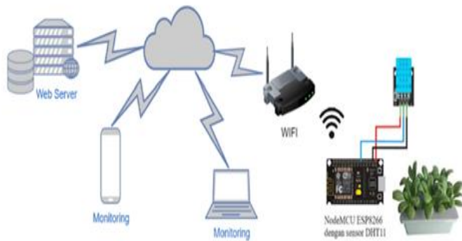
Fig. 6. Architecture for data collection and monitoring of hydroponic cultivation
