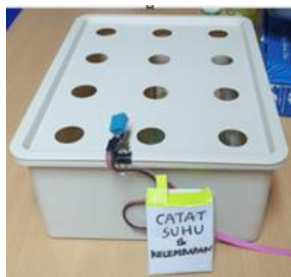
Fig. 7. DHT11 sensor and ESP8266 Node MCU wrapped
