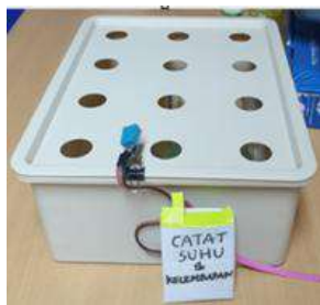
Fig. 7. DHT11 sensor and ESP8266 Node MCU wrapped
